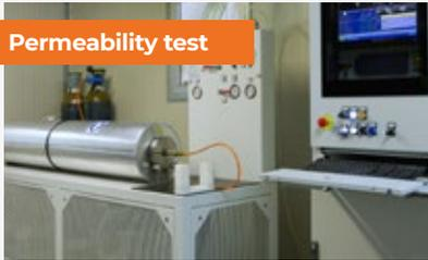
Permeability test of GOMAX QUADRA hoses according to EN 1736
