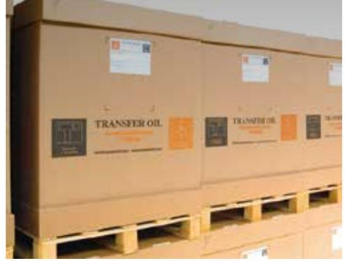
Special anti-humidity cardboard mounted on a ISPM 15 compliant Wooden Euro pallet 80 cm x 120 cm, in order to offer more reliable boxes during shipment both sea shipment and truck delivery.
